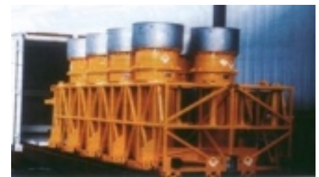
A 10 capacity rack with 8 FS47 flasks installed awaiting loading into the ISO container - note that the rack and flasks occupy virtually the whole of the ISO container cross section
