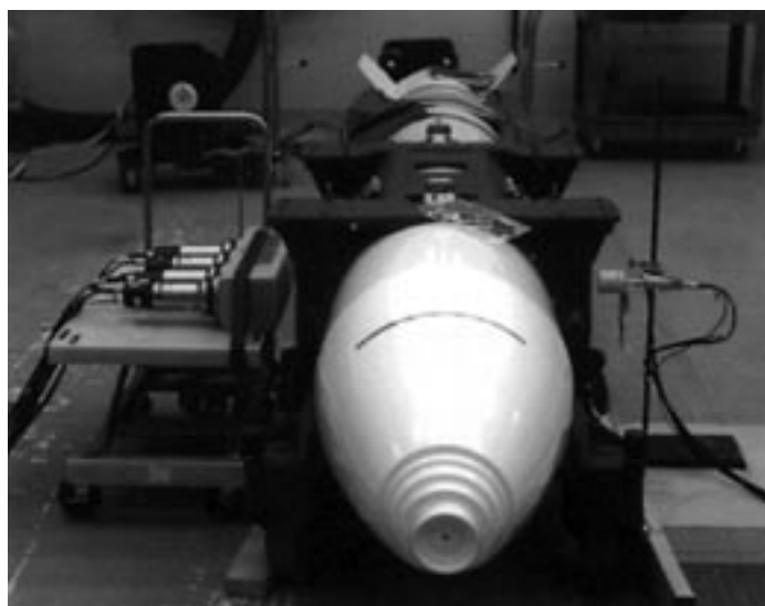
Figure 5.3 - The U.S. Nuclear Materials Identification System can measure the quantity and enrichment of HEU in a container or warhead. A weak source of neutrons on the right (one microgram or less of californium-252) irradiates the interior of an object – in this case a nuclear bomb – causing fissions in the HEU. The transmission
