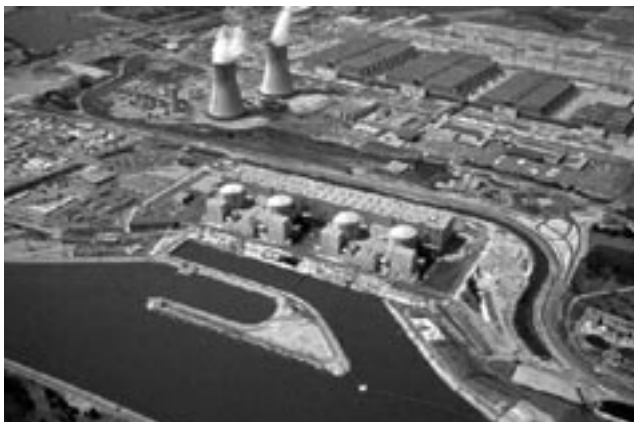
Figure 7.2 - France's Eurodif gas-diffusion uranium enrichment plant (large-area buildings in back) requires so much electrical power that it is co-located with a four-unit nuclear power plant. 169
