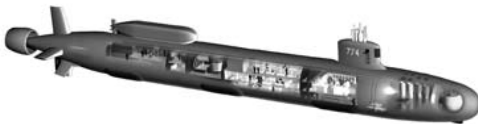
Figure 7.1. The new U.S. attack submarine (SSN-774, Virginia Class). The vessel uses highly enriched uranium in a lifetime core, i.e., does not require
